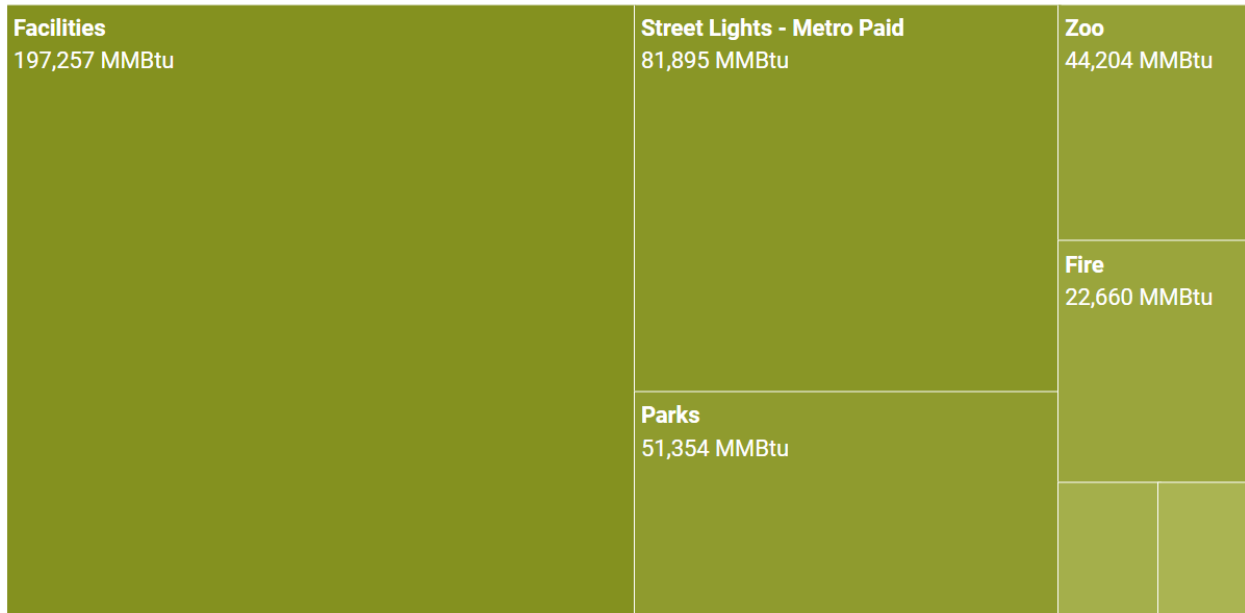
Figure 1: Breakdown of recorded energy usage by department. Departments managing numerous facilities have the highest associated energy usage, and street lighting is the largest consumer of power not associated with buildings.
